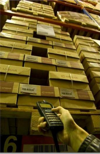
Picking of incoming and outgoing deliveries and inventory had to be conducted using barcodes and handheld terminals synchronised with a wireless network via a central server.
